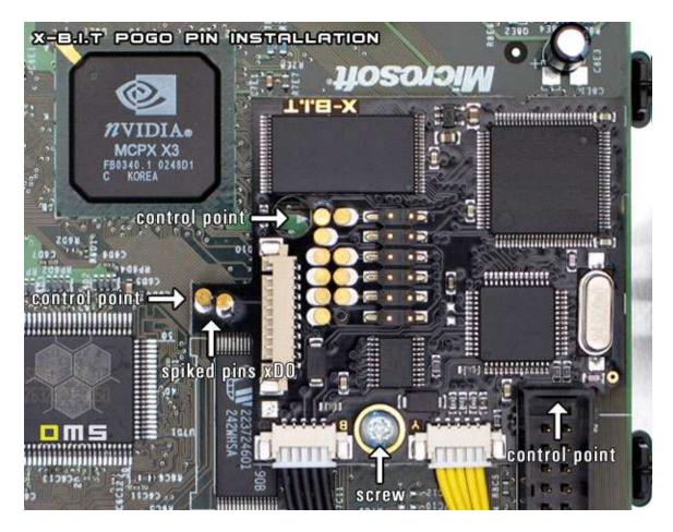
Position the X-B.I.T internal board by using the control points as shown above.
