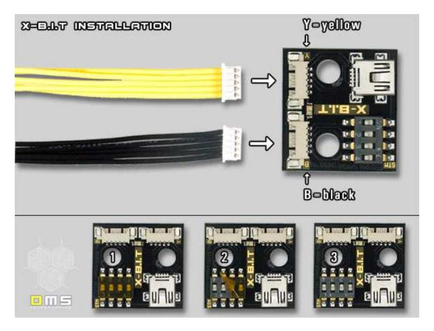
Connect the wires to the external board as shown above and ensure that you don't mix up the wires. Connect the yellow wires to the socket marked with "Y"and connect the black wires to the socket marked with "B". Remove the tape from the dip-switch.
