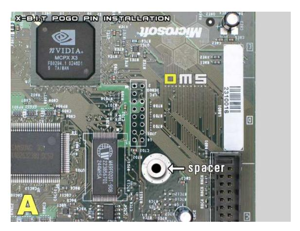
Remove the screw from the screw-hole shown above and position the spacer in the center of the screw-hole.
