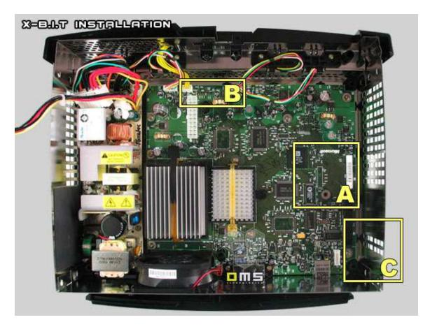
Remove the DVD-Drive and the HDD. You do not need to remove the XBox mainboard.
