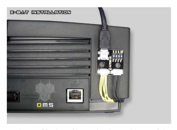
Route the wires carefully to the area of the XBox as shown above. Use adhesive-tape to fix the X-B.I.T external board on the back of the XBox. The physical installation is now completed.
