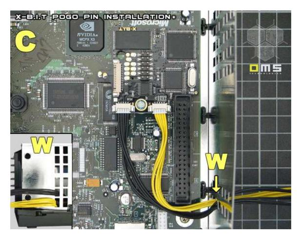
Route the wires carefully to the casing of the XBox and put them carefully through the cut-outs of the casing as shown above. The internal installation is now completed.
