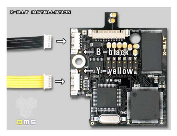
Connect the wires to the external board as shown above and ensure that you don't mix up the wires. Connect the yellow wires to the socket marked with "Y"and connect the black wires to the socket marked with "B".
