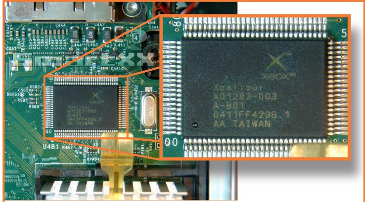
**5.** If the chip in your XBOX doesn't match the picture (Xcalibur marked on the chip): **DON'T FOLLOW THIS MANUAL ANY FURTHER!**
